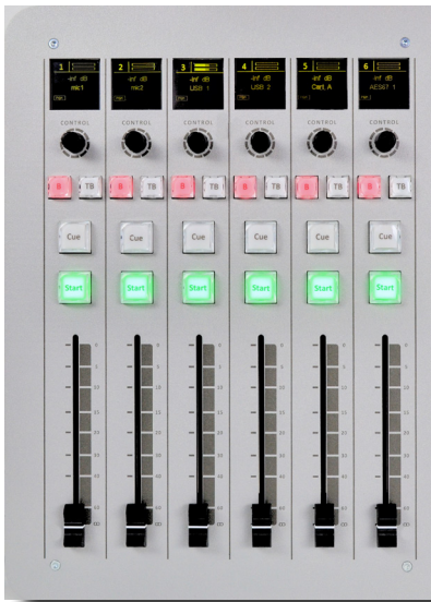
AXITE 6 fader Extender frame
